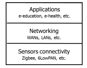
Fig. 1. Overall IOT Architecture
