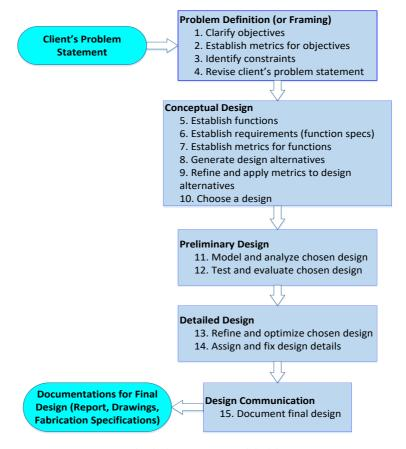
Fig. 1. The design process (modified from [8]).
