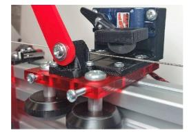
Fig. 9. Group I's string clamping system (note the compliant material.)
