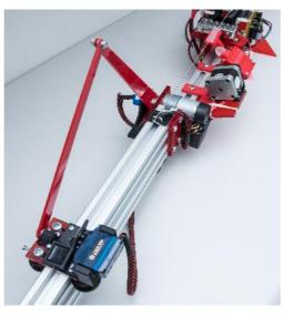
Fig. 8. Group I's SCARA arm pitch-shifting system
