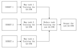
Figure 2. SVM algorithm based on MapReduce
