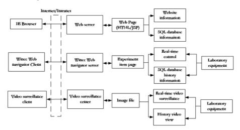
Fig. 1. Software structure of remote network teaching platform based on web server
