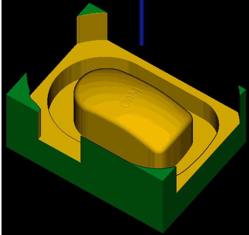
Fig. 3. Simulation result of punch machining
