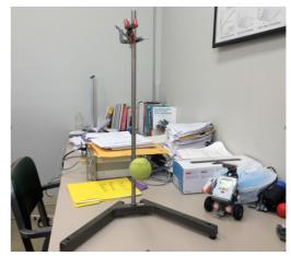
Figure 6. Experimental setup of Foucault pendulum
