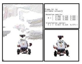
Figure 5. Complex object recognition; left: input point cloud; lower right: reference robot model; upper right: estimated motion
