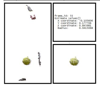
Figure 4. Scene with a spherical object; left: input point cloud after octree motion segmentation; lower right: result of RANSAC sphere detection; upper right: estimated sphere parameters
