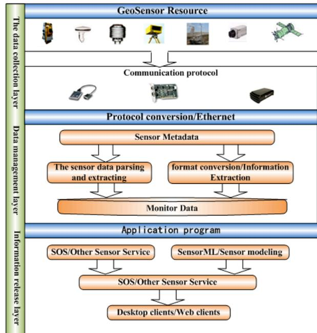
Figure 4. Multi sensor integration system framework for the ground disaster monitoring
