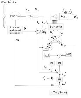
Figure 7 Control model of the generator
