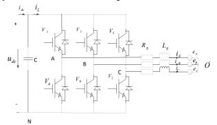
Figure 8 Direct-driven wind turbine grid side inverter
