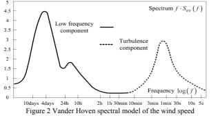
Figure 2 shows that the Vander Hoven wind speed spectrum model is composed of the mid-long term wind speed and the short-time wind speed (the part of the dotted line in Figure 2, the wind speed spectrum curve from the beginning of 10min to the right). The short-time wind speed is the main factor influencing the dynamic characteristics of the wind turbine and the wind energy capture efficiency. Therefore, The wind speed model established in the paper is the short-term wind speed model.
