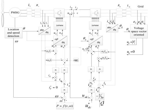
Figure 9 Direct-driven wind turbine machine side control system
