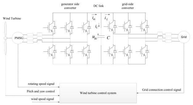
Figure 1 Overall structure of the direct-driven wind turbine
