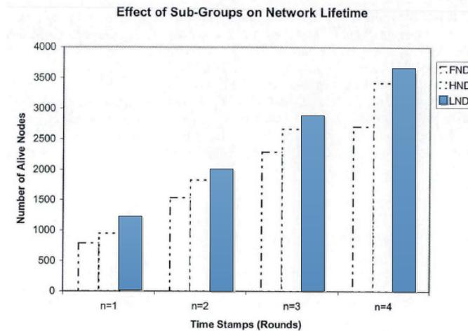
Figure 3. Pictographic of simulation for effect of sub-groups on network lifetime in MG-LEACH
