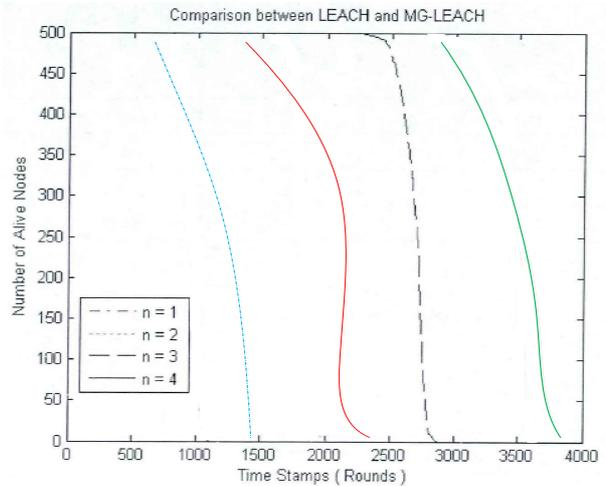
Figure 2. Graphical representation of simulation results presenting effect of creating different sub-groups on network lifetime
