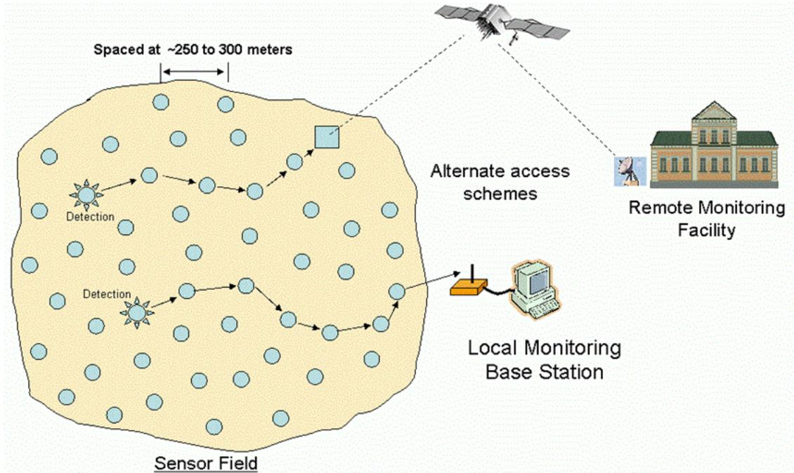
Figure 1. The wireless sensor network tree topology
