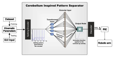
Fig. 4. Cerebellum Inspired Pattern Separator for GUI based Remote labs
