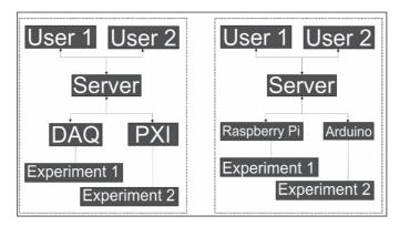
Fig. 2. Remote lab deployments with proprietary (left) and open-source implementations (right).
