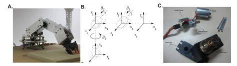
Fig. 1. Deploying a low-cost robotic arm as a remote lab: A. 6 DOF robotic manipulator used as an equipment for remote lab B. Axis representation for the joint angles. C. Servo motor components
