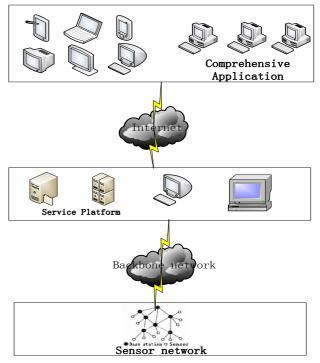
Figure 1. Internet of things mine safety online detection system architecture
