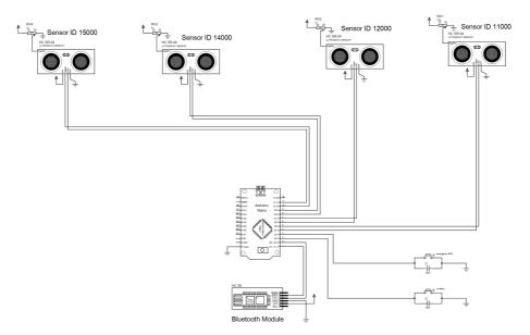
Fig. 2. Simulation of the blind stick via Proteus 8.0
