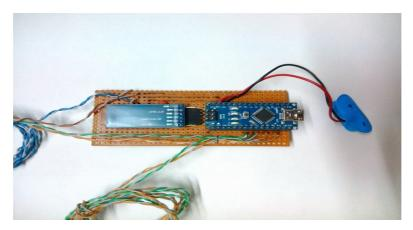
Fig. 5. Bluetooth module connection of the stick
