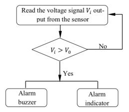
Fig. 7. Flow chart of refitted part of ECU program
