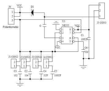
Fig. 3. Data conversion module of tilt sensor
