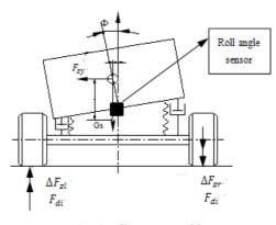
Fig. 6. Tilt sensor position
