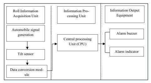
Fig. 1. Block diagram of roll warning system
