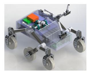
Fig. 6. CAD model of the robot manipulator VALI-3
