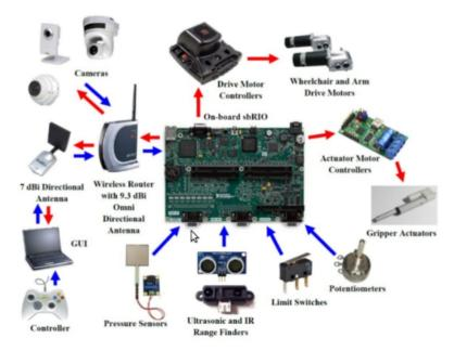
Fig. 2. Electronic robot architecture of the Worcester Polytechnic Institute
