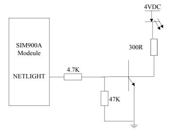
Fig. 4. Network status indication circuit
