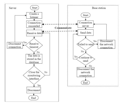
Fig. 3. The specific flow of the two-machine communication
