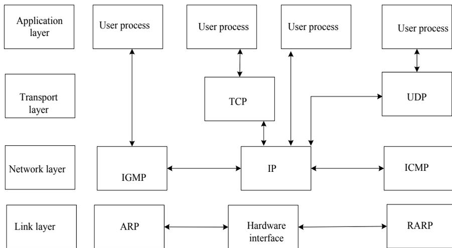
Fig. 3. TCP / IP protocol structure model
