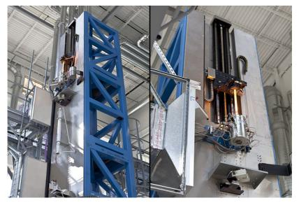
Fig. 5. Glass preform being fed into the draw furnace, Thorlabs [7]
