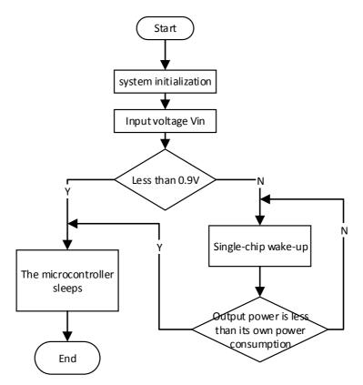
Fig. 2. Flow Chart of Power Supply Control Software
