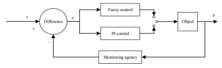
Fig. 1. Fuzzy-PI Dual Mode Control System Structure
