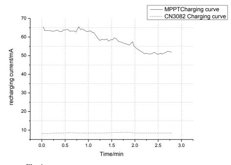
Fig. 4. Contrast Experimental Data between MPPT Charging and CN3082 (non-MPPT) Charging
