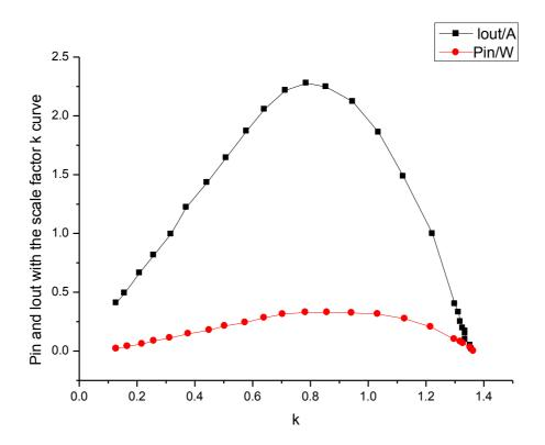
Fig. 3. Curve of Solar Panel Input Power Pin and DCDC Circuit Output Current Lout Changing with k
