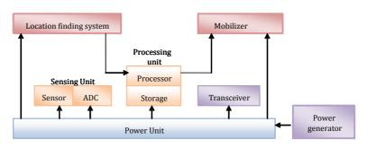
Fig. 2. Nodes and data processing architecture of WSN
