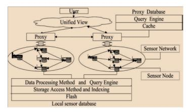
Fig. 1. Wireless Sensor Network Database System Architecture
