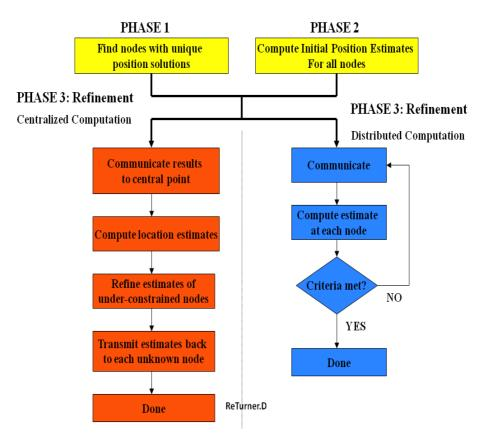
Fig. 6. Workflow of self-localization algorithms
