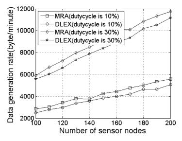
Fig. 1. Data generation rate with number of nodes increasing when duty cycle is 10% and 30%
