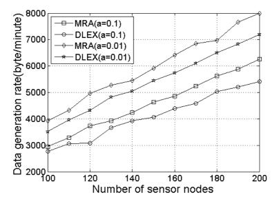
Fig. 2. Data generation rate with number of nodes increasing when data correlation  $\alpha = 0.01, 0.001$
