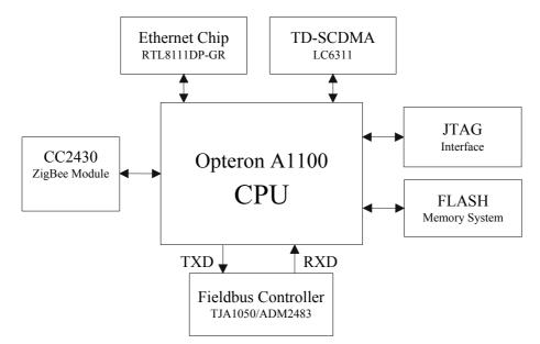
Fig. 2. IOT Gateway Hardware Structure Diagram of the System Platform
