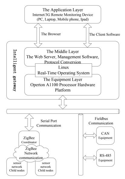
Fig. 1. IOT System Overall Structure
