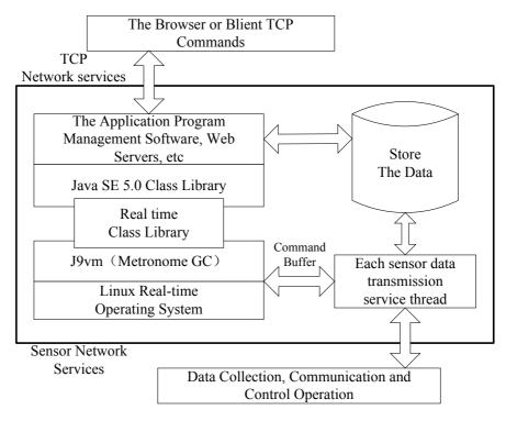
Fig. 3. IOT Gateway Software Hierarchy Structure
