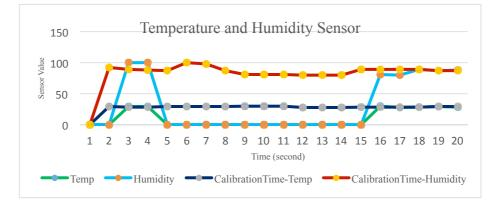
Fig. 6. The result of calibration time for temperature and humidity sensing element.
