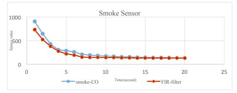
Fig. 7. Self-calibrate by FIR filter.
