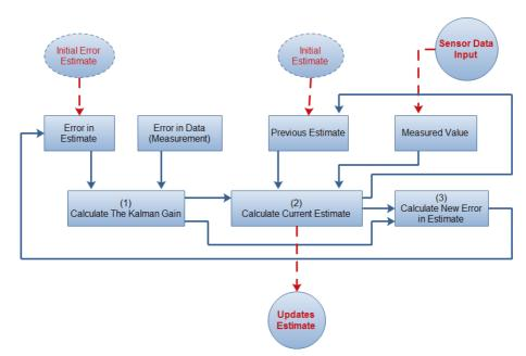
Fig. 2. The FSKF diagram with sensors data input.
