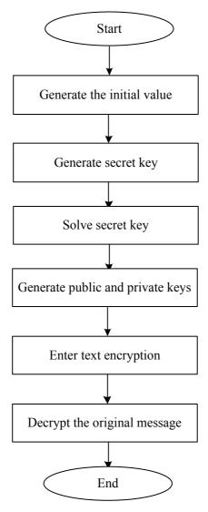
Fig. 4. RSA algorithm flow chart
