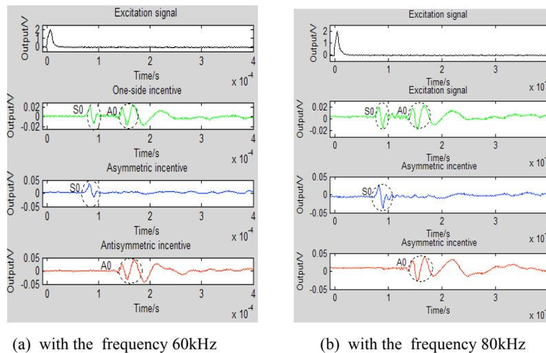
Fig. 8. Response of detection point A at different frequencies
