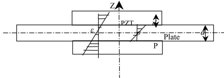
Fig. 2. Excitation principle diagram of double piezoelectric wafers
