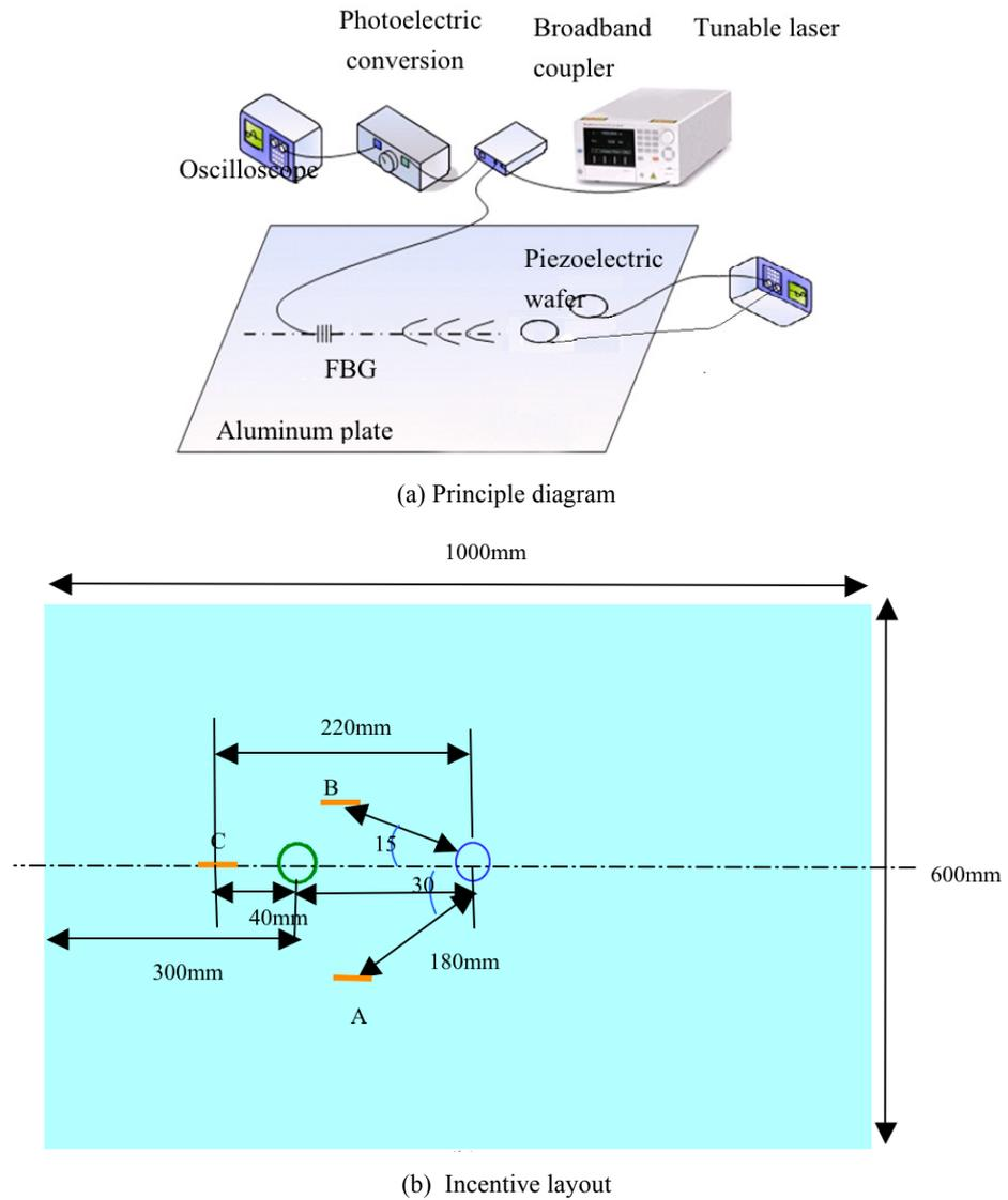
Fig. 6. xperimental equipment
