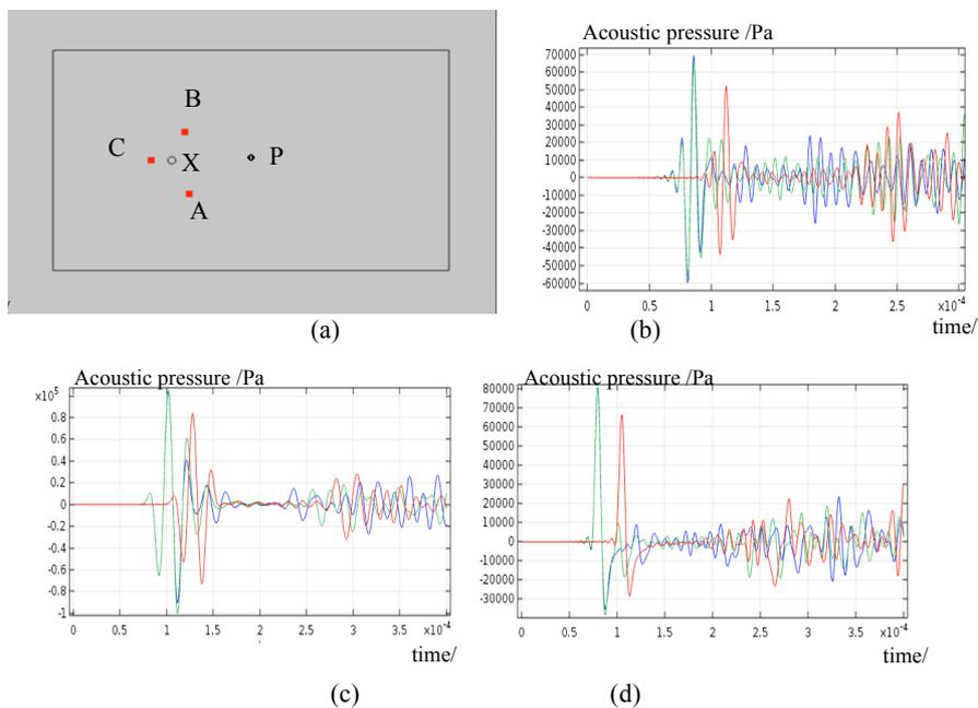
a- Monitoring point arrangement ; b-Three peak modulation wave with 100kHz;
