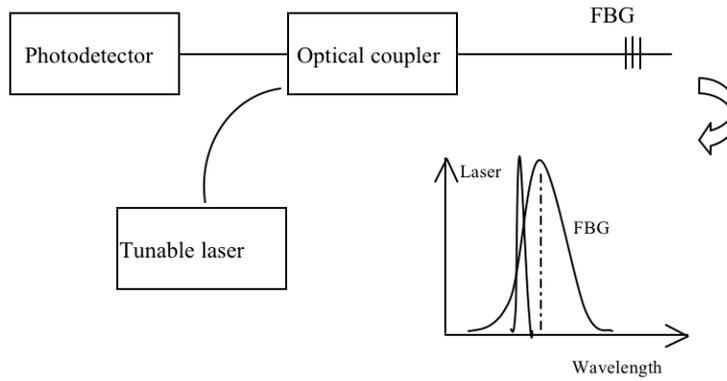
Fig. 3. The demodulation principle of FBG sensor
