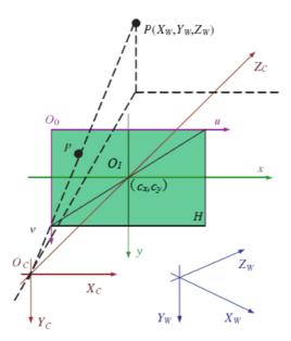
Fig. 7. The imaging model of 3D image
