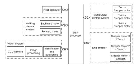
Fig. 3. The circuit control frame diagram of target fruit recognition system
