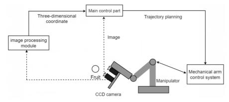
Fig. 2. The schematic diagram of the fruit recognition system for the target of the picking robot
