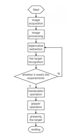
Fig. 4. The schematic diagram of the software flow of the intelligent picking robot system
