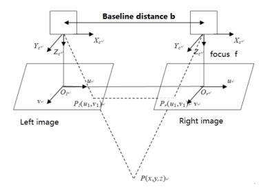
Fig. 8. Fig.8 The schematic diagram of the principle of binocular vision positioning
