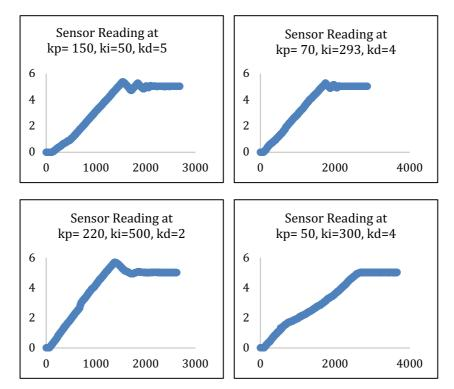
Fig. 5. The results of the evaluation of PID controller's performance from the plant console
