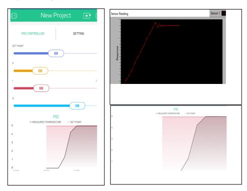
Fig. 4. Remote console interface of temperature control systems
