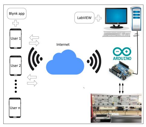
Fig. 1. The architecture of the remote laboratory
