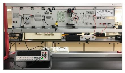
Fig. 2. The plant console of LD-Didactic equipment's temperature control
