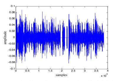
Fig. 2. I-channel time domain waveform of LTE downlink baseband signal
