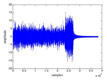
Fig. 6. DST transform coefficient distribution diagram of I-channel sampling of LTE downlink baseband signal
