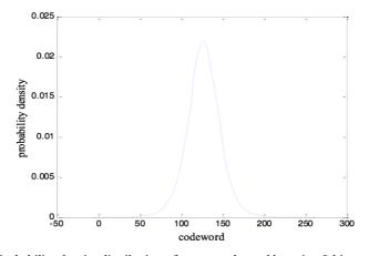
Fig. 8. Probability density distribution of output codeword by using 8-bit quantization
