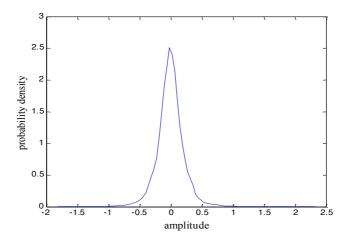
(b) Probability density distribution diagram of low energy block coefficients
