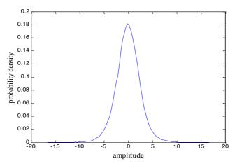
(a) Probability density distribution diagram of high energy block coefficients
