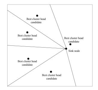
Fig. 5. The case when the sink node moves to the edge of the network
