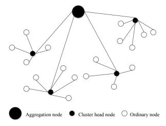
Fig. 1. Wireless sensor network architecture under LEACH protocol
