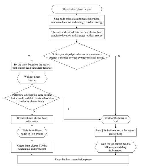
Fig. 3. The workflow of clustering structure construction phase in M-LEACH protocol
