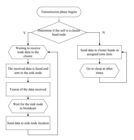
Fig. 4. Packet transmission phase work flow in M-LEACH protocol
