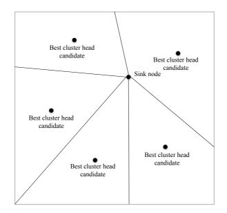
Fig. 2. M-LEACH protocol network partition and "best cluster head candidate position" schematic diagram
