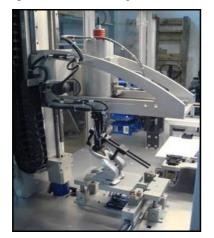
Figure 5. The testing bench of staplers and perforators to repair
