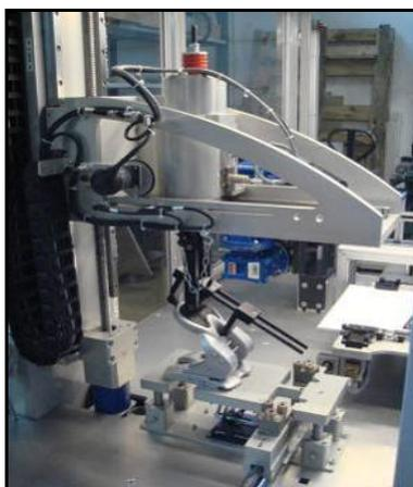
Figure 5. The testing bench of staplers and perforators to repair
