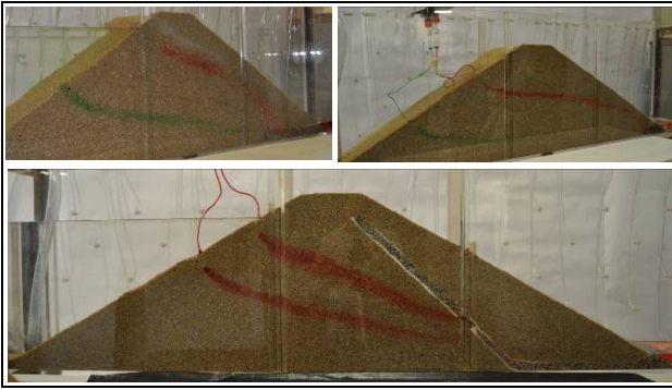
Figure 6. Flow lines in a dam with drainage blanket, toe drain and chimney drain (clockwise from top left)
