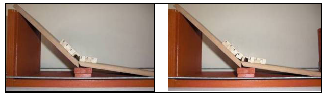
Figure 10. Initial state (left) and new equilibrium configuration after instabilization
