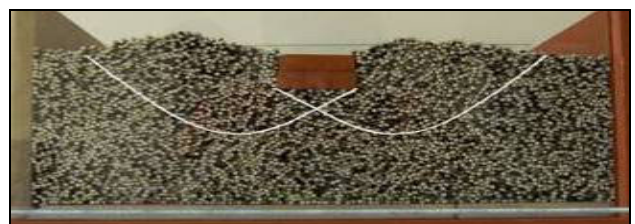
Figure 12. Failure mechanism of a small scale shallow foundation
