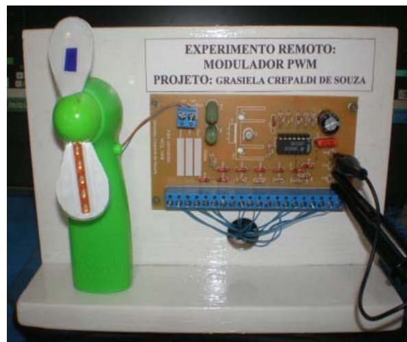
Figure 15. Ventilator connected to the PWM modulator remote experiment via internet
