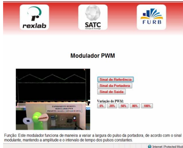
Figure 14. PWM remote experiment via internet
