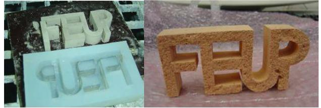
Figure 5. Silicone mould and decorative ceramic part cast on it.
