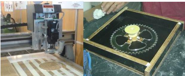
Figure 3. Ceramic block moulding to cast a duraluminium gear.
