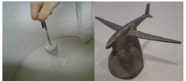
Figure 6. Metallic airplane for tests in a wind tunnel; CAD model, quick cast model, ceramic shell manufacturing and metallic casted part.
