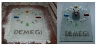
Figure 2. Glass fusing technique to manufacture a wall clock. The white powder is a demolding agent (boron nitride).
