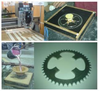
Figure 3. Ceramic block moulding to cast a duraluminium gear.
