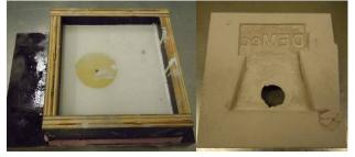
Figure 8. Box containing the model with the gating system and the slurry, and final ceramic mould with defects.
