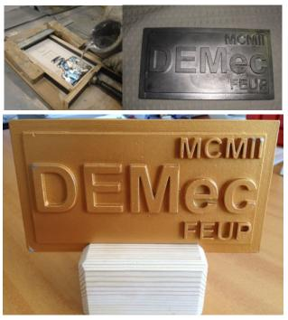
Figure 11. Casting the low melting point alloy and final part.
