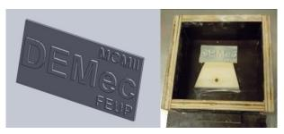
Figure 7. Image of the metallic plate to be obtained and SL prototype with the gating system.
