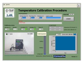
Figure 3. Temperatura calibration procedure remotely accessible: user interface.
