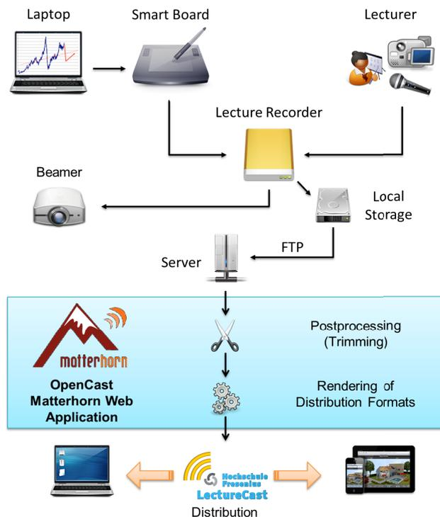
Figure 3. Schematic View of the Lecture Recording System and Workflow
