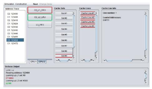
Figure 9. Overview of simulation mode of EDUCache simulator, L1 miss and L2 hit while reading the address 123464
