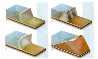
Figure 1. A – Gravity dam; B – Buttress dam; C – Arch dam; D – Embankment dam (adapted from [3]).
