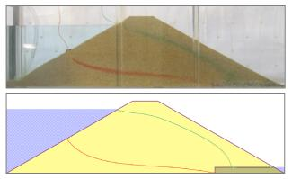
Figure 5. Experimental and numerical results for flow line configuration in small scale dam with toe drain.
