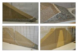
Figure 4. Drainage blanket, toe drain, clay core and chimney drain (clockwise from top left).
