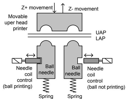
Figure 9. The printer head.
