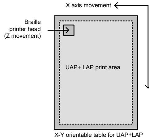
Figure 6. The principle of the XYZ table from the stereotype machine.
