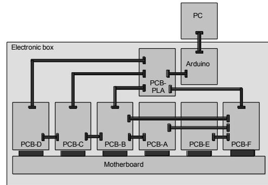
Figure 11. The new PCBs scheme on the electronic box and the PC connection.
