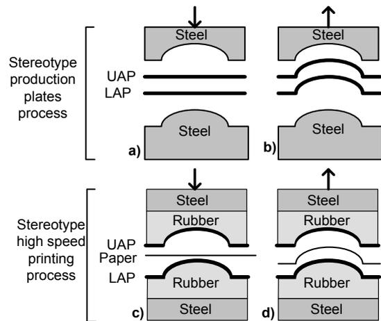
Figure 4. The stereotype production scheme.
