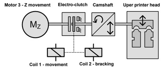
Figure 10. The Z movement generation.
