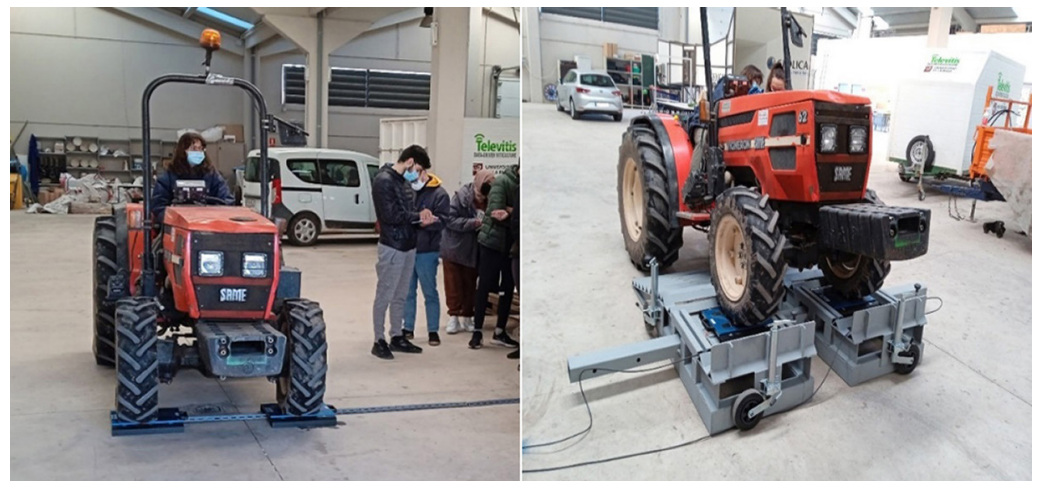
Fig. 3. Tractor weighing process: (left) the tractor on a flat surface to determine the center of gravity location between the two axles; (right) the tractor on the ramps to determine the height of the center of gravity
