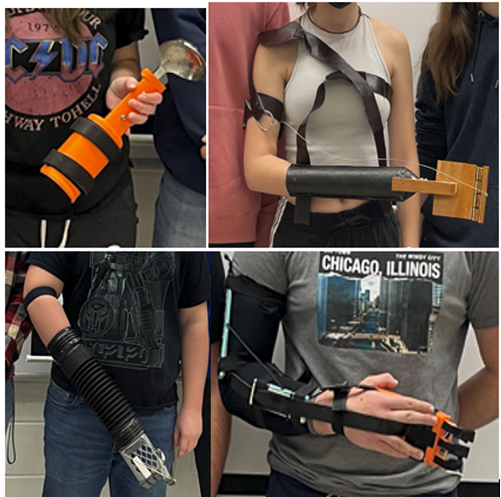
Fig. 1. Examples of student team products. Teams were tasked to design and construct a prototype trans-radial prosthetic arm for children
