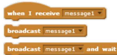
Figure 6. Blocks for sending and receiving messages
