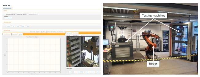
Figure 4. Remote laboratory at IUL: Lab Client (left) and testing cell (right) [4]
