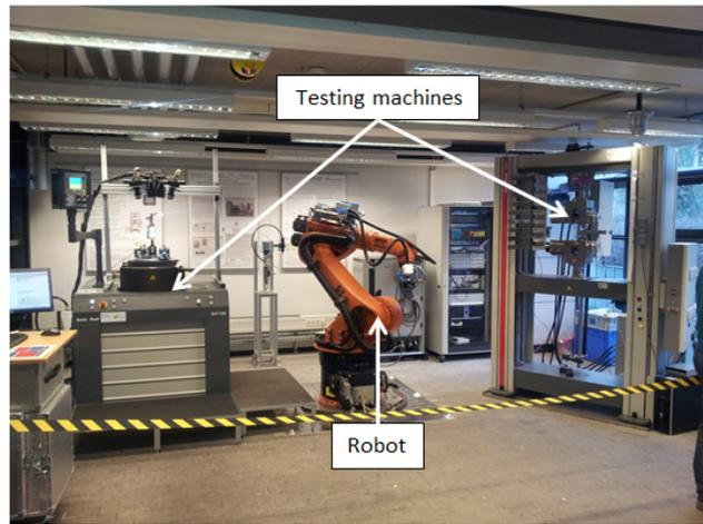
Figure 4. Remote laboratory at IUL: Lab Client (left) and testing cell (right) [4]
