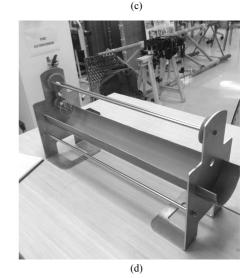
Figure 2. (a) Cassava crackers sold in local market. (b) Manual cassava juice extracting method; two workers squeeze the juice by twisting the sack filled with shredded cassava in opposite directions (c) CAD design of envisioned device where same motion is done by rotating the handles on both sides in opposite directions generating squeeze motion. Handle and gear mechanism makes the job less strenuous (d) Final
