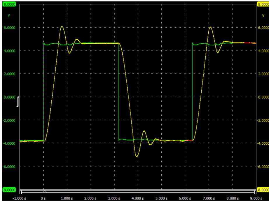
**Fig. 10.** Output response with ringing (microcontroller-based controller,  $K_p=25$  and  $K_v=0$ )
