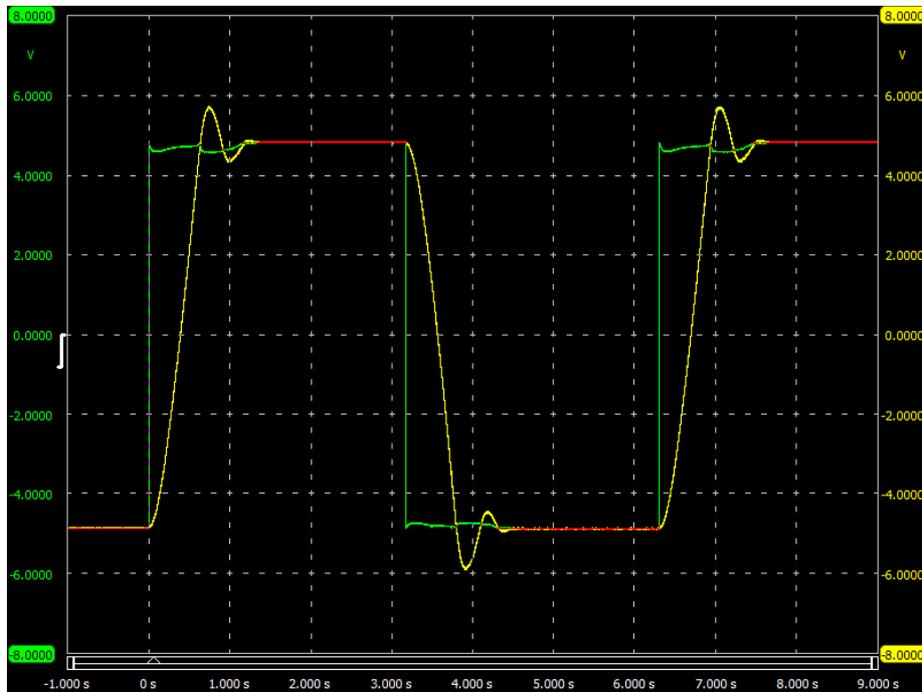
Fig. 4. Output response with ringing (op amp-based controller)
