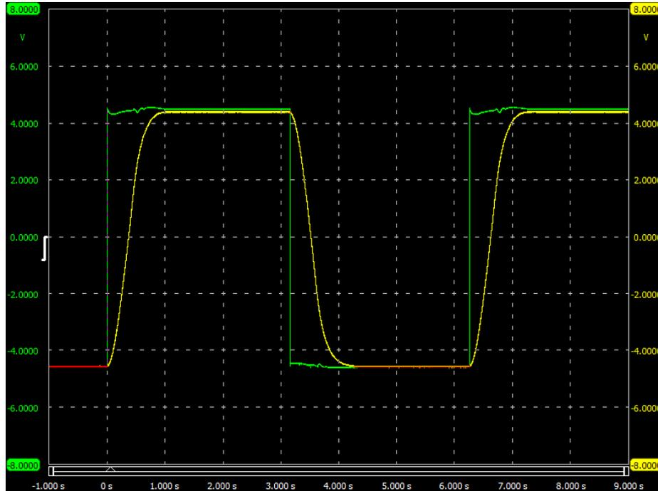
Fig. 8. Output response with ringing removed by velocity feedback (op amp-based controller)
