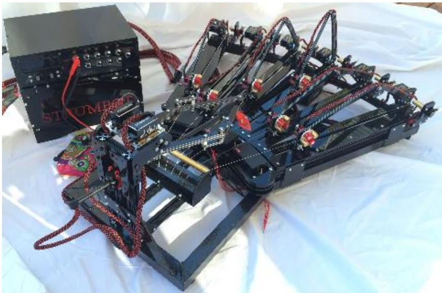
**Fig. 3.** StrumBot – an integrated six-string guitar [18]
