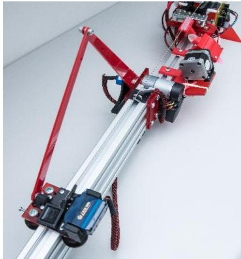
**Fig. 8.** Group I's SCARA arm pitch-shifting system
