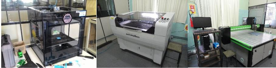
**Fig. 3.** RP equipment to develop PBL classes (3D Printer, Laser cutting machine and Milling Router).
