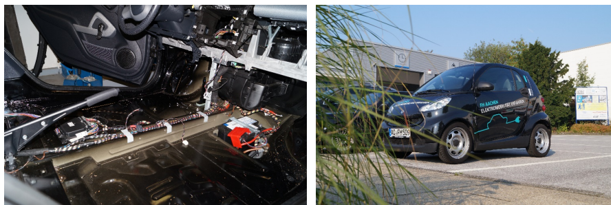
Fig. 6. Conversion of the Smart to an E-Smart: new harness (left) and E-Smart after official approval (right)
